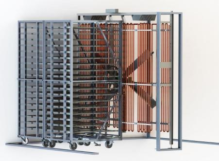
Trolleys orientated to allow efficient airflow through eggs
