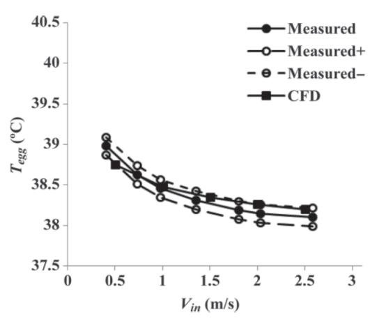
Figure 9. The average eggshell temperature,  $T_{egg}$ , versus inlet air velocity,  $V_{in}$ , for horizontal flow with an ambient temperature  $(T_{amb}) = 37.70^{\circ}$ C and a heat production of the egg  $(Q_{egg}) = 148.5 \text{ mW}$ , as simulated with computational fluid dynamics (CFD) and measured by Van Brecht (2004). Measured = average value; Measured  $\pm$  = average value  $\pm$  accuracy of the thermocouple  $\pm$  SD of measured values.
