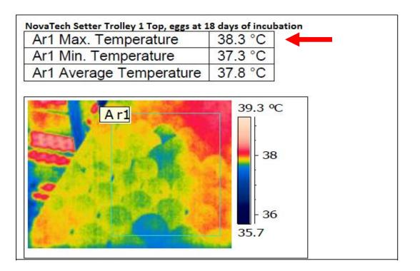
Thermal Image of a tray of eggs showing the egg shell temperatures with embyros at 18 days of incubation from the new NovaTech Setter, same trolley and position – Trolley 1 – Top. Note that the temperatures are within the ideal range of between 37.8°C and 38.3°C. The blue colour would be indicative of infertile eggs
