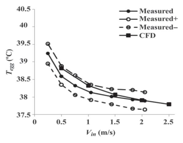
Figure 3. The average eggshell temperature,  $T_{egg}$ , versus inlet air velocity,  $V_{in}$ , for horizontal flow with an ambient temperature  $(T_{amb}) = 37.36^{\circ}$ C and a heat production of the egg  $(Q_{egg}) = 285.6 \text{ mW}$ , as simulated with computational fluid dynamics (CFD) and measured by Van Brecht et al. (2005). Measured = average value; Measured  $\pm$  average value  $\pm$  accuracy of the thermocouple  $\pm$  SD of measured values.
