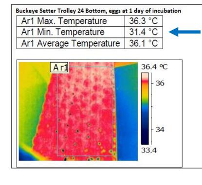
Thermal image from a Buckeye Setter, trolley 24 bottom, looking at eggs freshly set and only 1 day into incubation, shows a minimum temperature of only 31.4°C and has an average temperature of 36.1°C with a maximum temperature of only 36.3°
