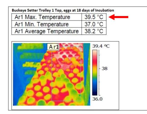
Thermal Image of a tray of eggs showing the egg shell temperatures with embyros at 18 days of incubation from a 10 year old Buckeye Setter, from the top of Trolley 1 (first trolley from the front on the left). Note temperatures in excess of 39.4°C, which can be detrimental to chick quality. The lighter yellow and green are likely to be indicative of infertile eggs.
