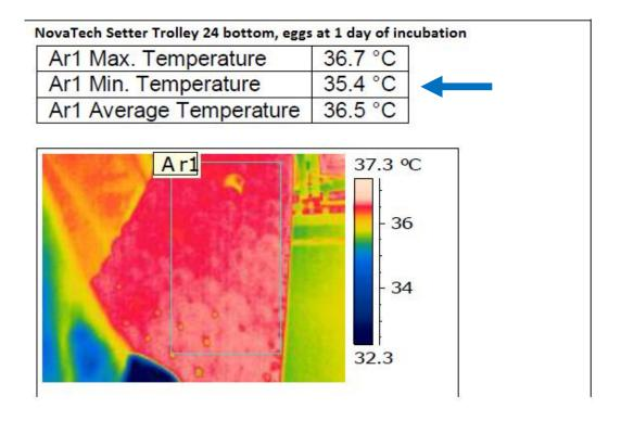
Thermal image from the NovaTech Setter trolley 24 bottom, note the much higher temperatures, showing a minimum temperature of 35.2°C, an average temperature of 36.5°C and a maximum temperature of 36.7°2
