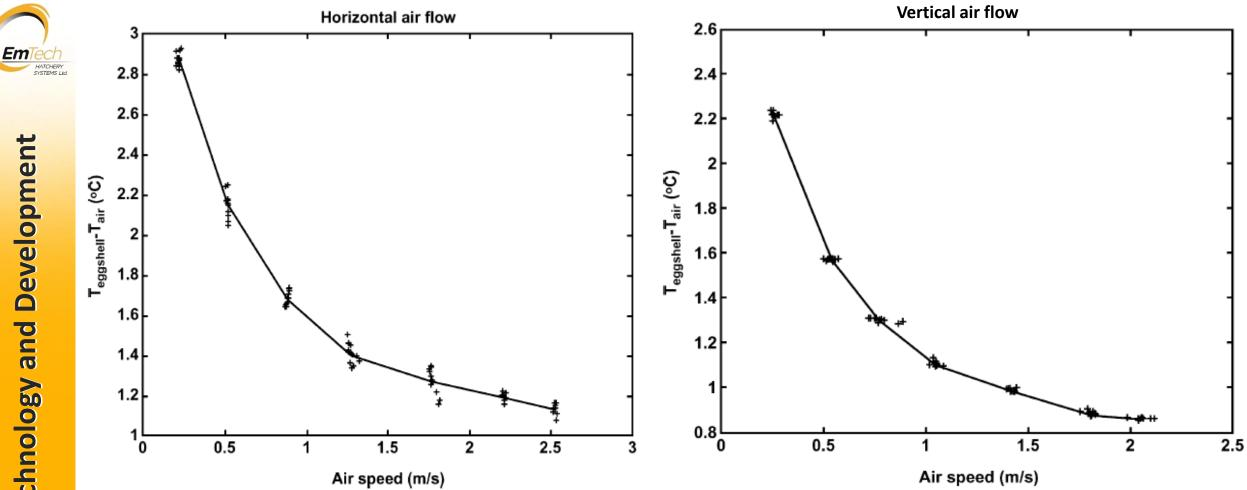
FIGURE 6. The temperature difference between the air and the eggshell as a function of the air speed of a horizontal airflow at 285.6 mW of sensible heat production.
